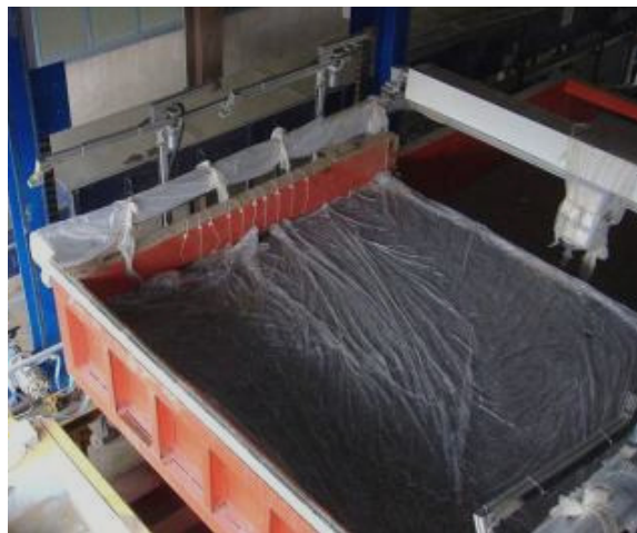
Figure 10. Rest position of rain simulation system.
