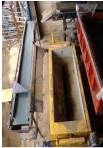
Figure 7. The conveyer belt used to spread soil into the hopper.
