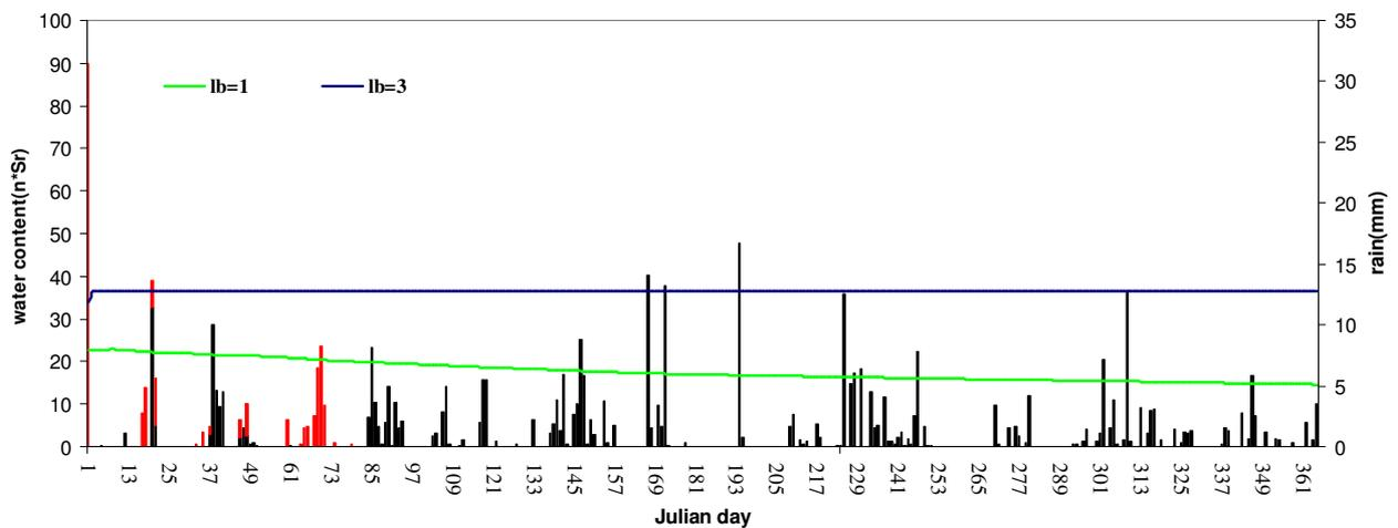
**graph 31:** the black bar represents the cumulated daily precipitations; the red bar represents the snow precipitation; the others bars are the soil moisture curves in the VII layer varying the lower boundary (green line for the unit gradient condition and blue for constant groundwater condition)
