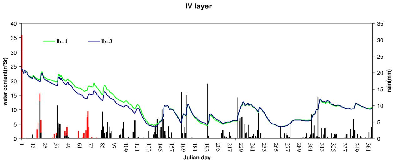
**graph 29**: the black bar represents the cumulated daily precipitations; the red bar represents the snow precipitation; the others bars are the soil moisture curves in the IV layer varying the lower boundary (green line for the unit gradient condition and blue for constant groundwater condition)
