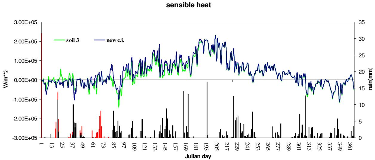
**graph 26:** the black bar represents the cumulated daily precipitations, the red bar represents the snow precipitation; the others bars are the sensible heat curves varying the initial conditions (green line for old i.c., blue for new i.c)
