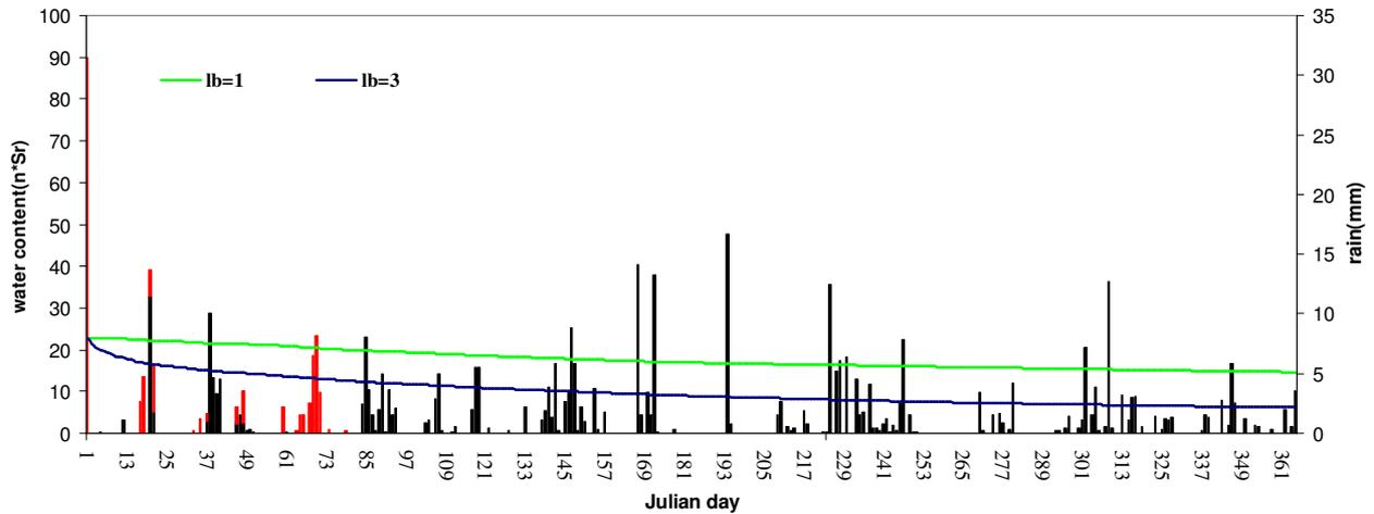
**graph 30:** the black bar represents the cumulated daily precipitations; the red bar represents the snow precipitation; the others bars are the soil moisture curves in the VI layer varying the lower boundary (green line for the unit gradient condition and blue for constant groundwater condition)
