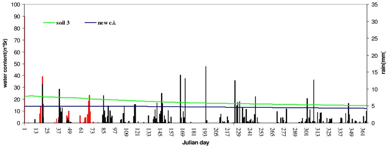
**graph 22:** the black bar represents the cumulated daily precipitations, the red bar represents the snow precipitation; the others bars are soil moisture curves in the VIII layer varying the initial conditions (green line for old i.c., blue for new i.c)
