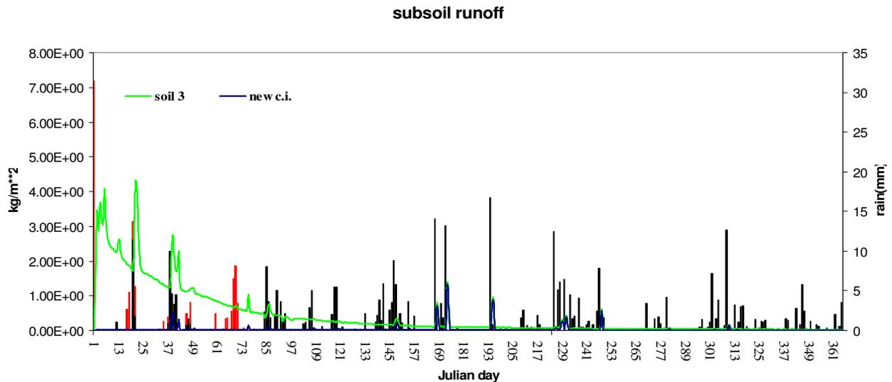
**graph 27:** the black bar represents the cumulated daily precipitations, the red bar represents the snow precipitation; the others bars are the subsoil runoff curves varying the initial conditions (green line for old i.c., blue for new i.c)
