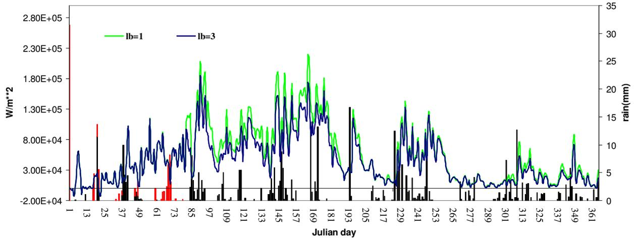
**graph 32** the black bar represents the cumulated daily precipitations; the red bar represents the snow precipitation; the others bars are latent heat curves varying the lower boundary (green line for the unit gradient condition and blue for constant groundwater condition)
