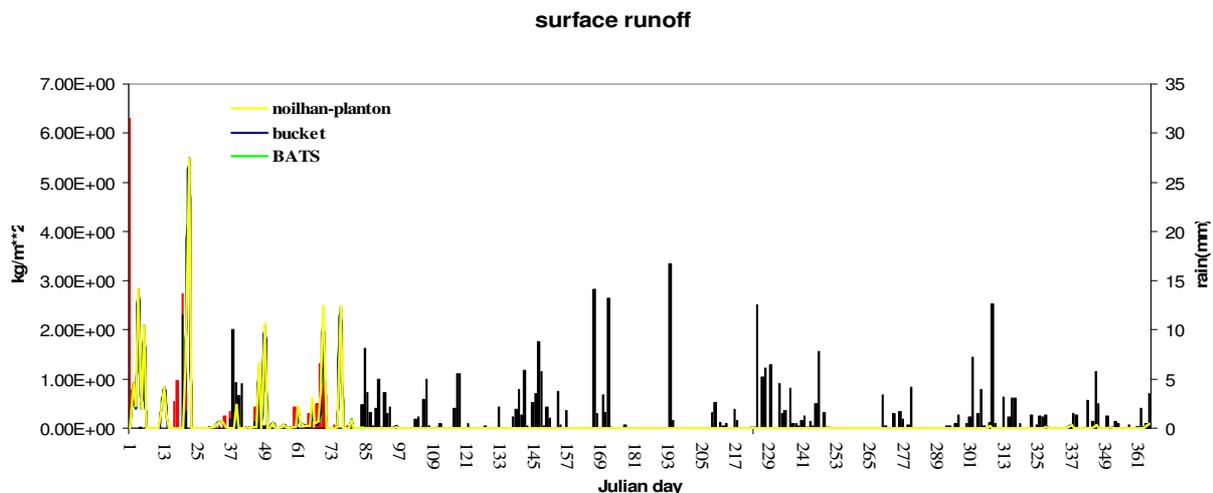
**graph 18:** the black bar represents the cumulated daily precipitations, the red bar represents the snow precipitation; the others bars are the surface runoff curves varying the evaporation model (green line for BATS model, yellow line for Noilhan-Planton model and blue for bucket model)
