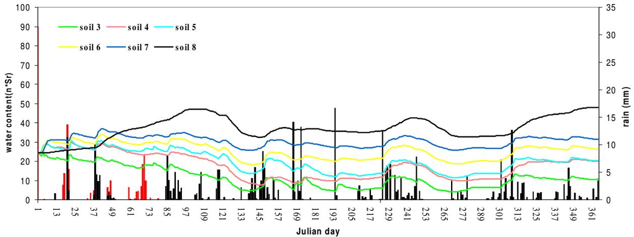
**graph 4:** : the black bar represents the cumulated daily precipitations and the red bar represents snow precipitation; the others curves are the water content curves in the IV soil level varying the soil type
