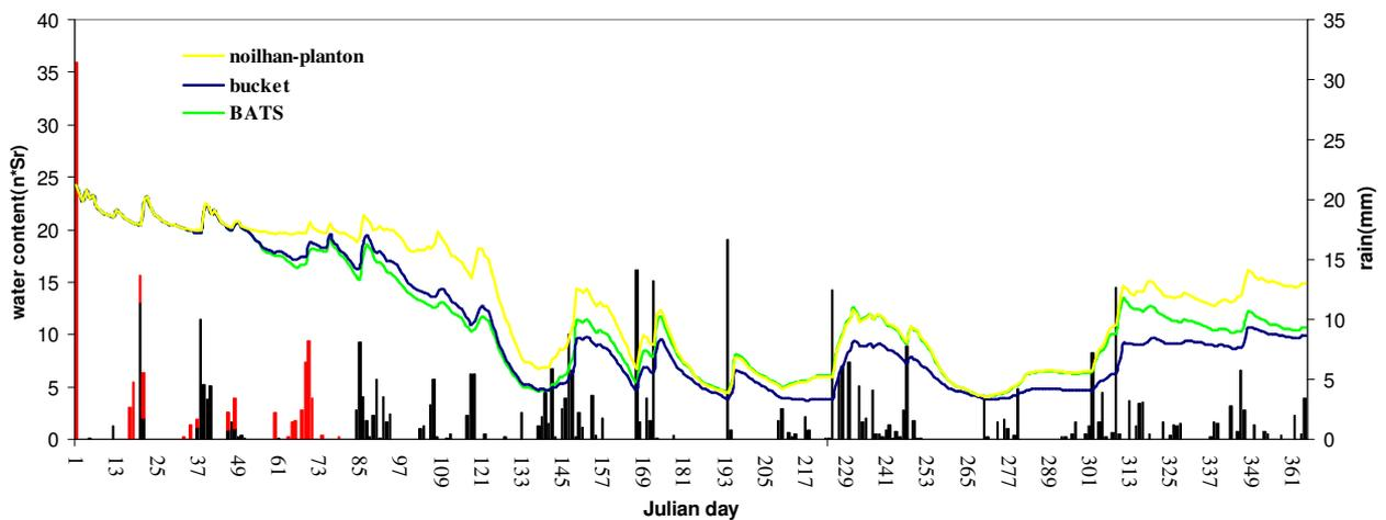
**graph 14:** the black bar represents the cumulated daily precipitations, the red bar represents the snow precipitation; the others bars are the soil moisture curves in the IV layer varying the evaporation model (green line for BATS model, yellow line for Noilhan-Planton model and blue for bucket model)
