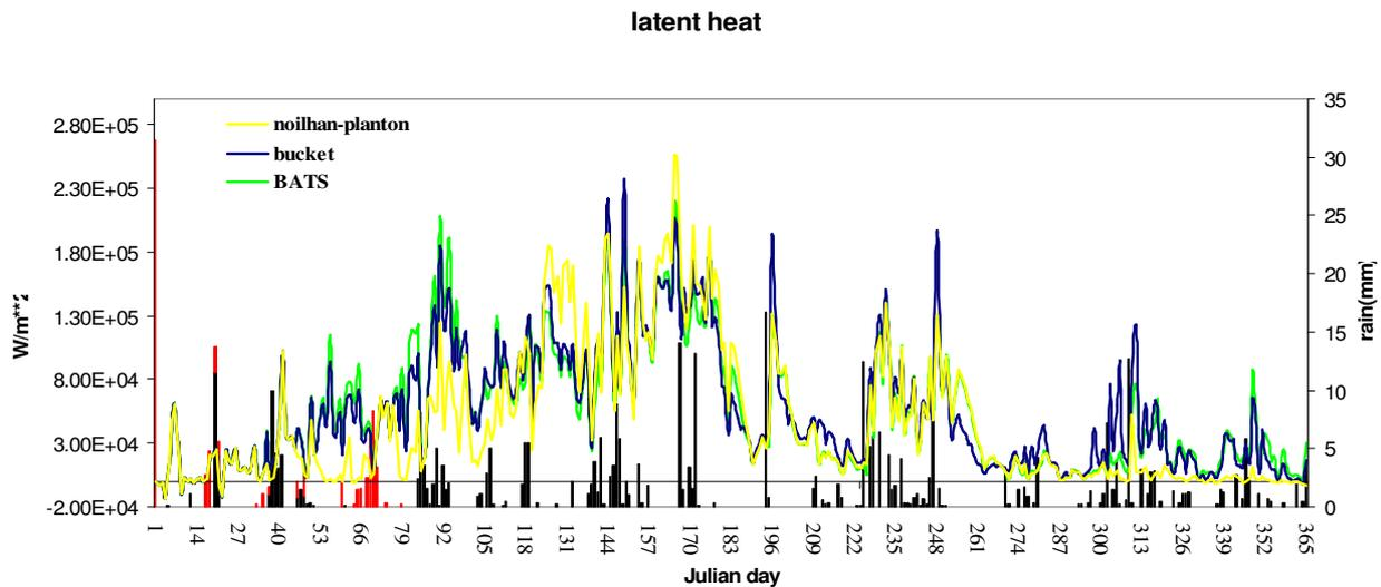
**graph 17:** the black bar represents the cumulated daily precipitations, the red bar represents the snow precipitation; the others bars are the latent heat curves varying the evaporation model (green line for BATS model, yellow line for Noilhan-Planton model and blue for bucket model)
