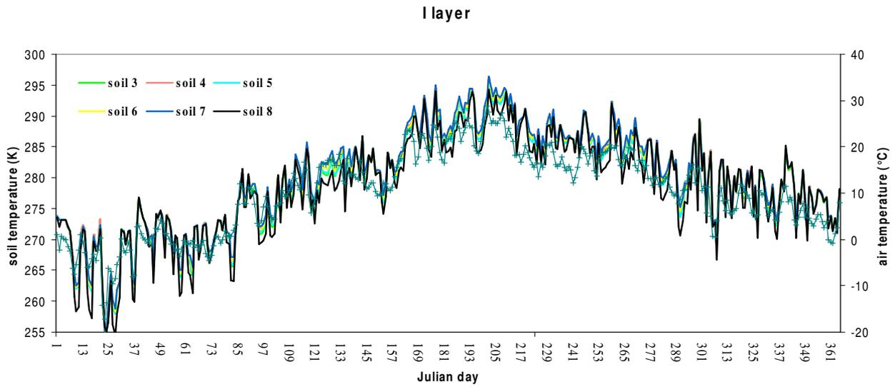
**graph 6:** the grey curve with the crosses represents the air temperature; the others curves are the soil temperature curves in the first soil level varying the soil type
