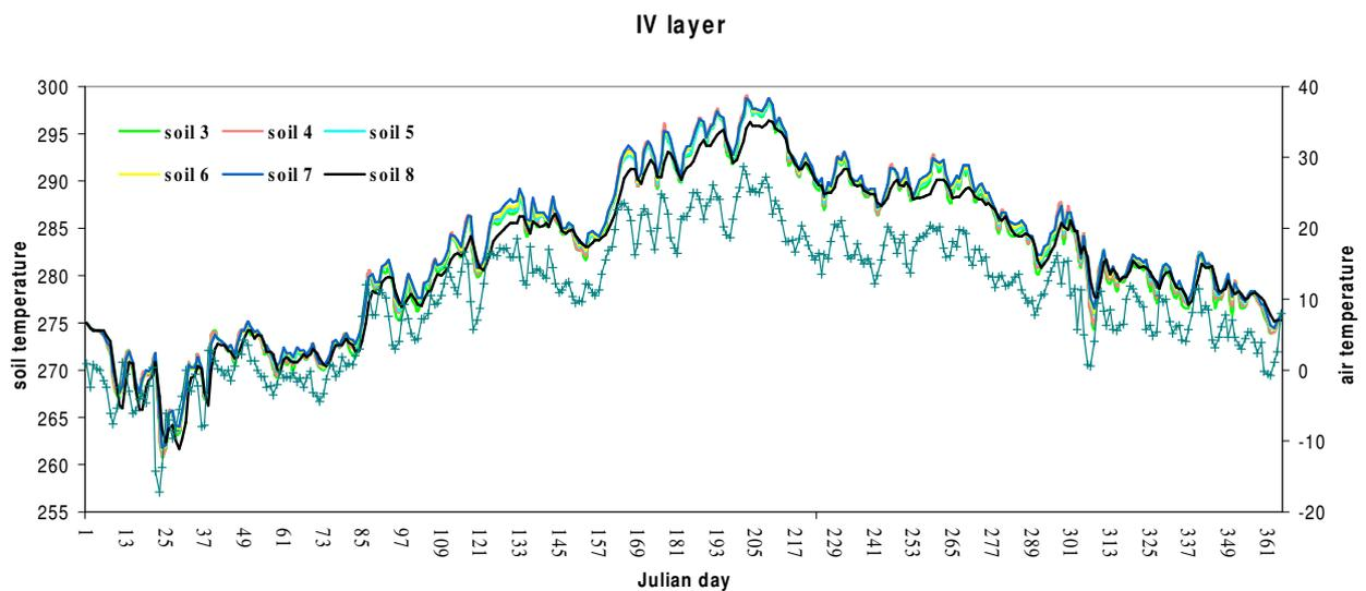
**graph 7:** the grey curve with the crosses represents the air temperature; the others curves are the soil temperature curves in the IV soil level varying the soil type
