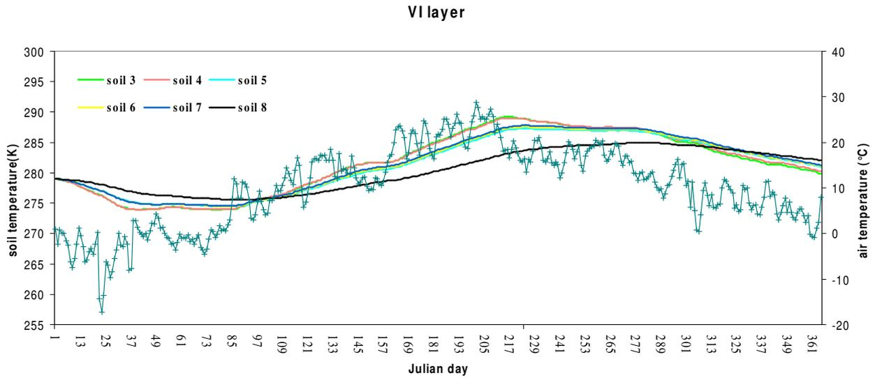
**graph 8:** the grey curve with the crosses represents the air temperature; the others curves are the soil temperature curves in the VI soil level varying the soil type
