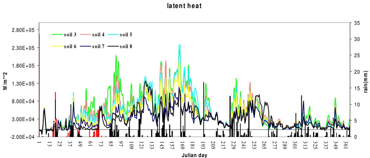
**graph 9:** the black bar represents the cumulated daily precipitations and the red bar represents snow precipitation; the others curves are the latent heat curves varying the soil type
