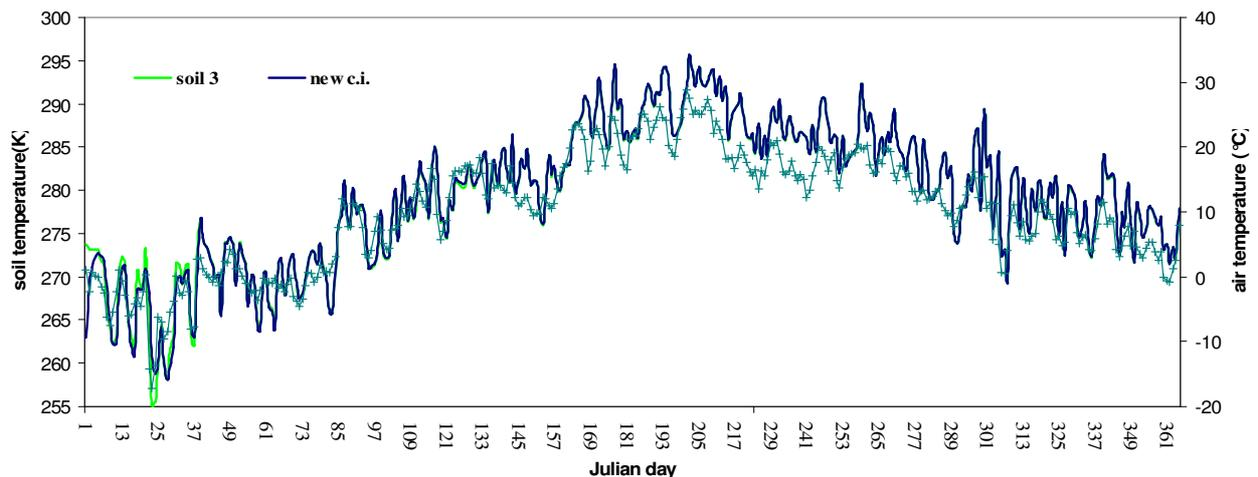
**graph 23:** the grey curve with the crosses represents the air temperature; the others bars are the soil temperature curves in the I layer varying the initial conditions (green line for old i.c., blue for new i.c)
