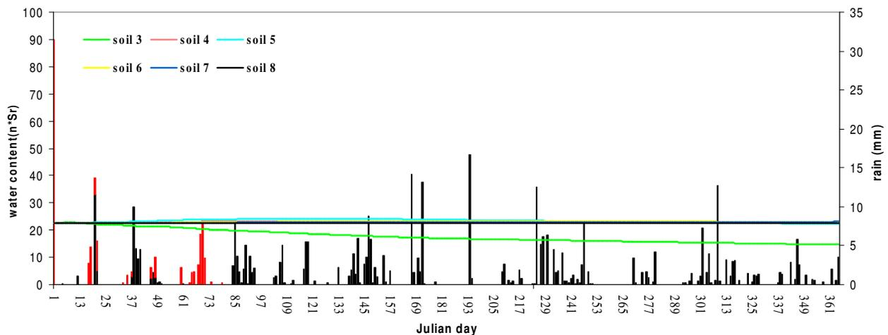
**graph 5:** : the black bar represents the cumulated daily precipitations and the red bar represents snow precipitation; the others curves are the water content curves in the VIII soil level varying the soil type
