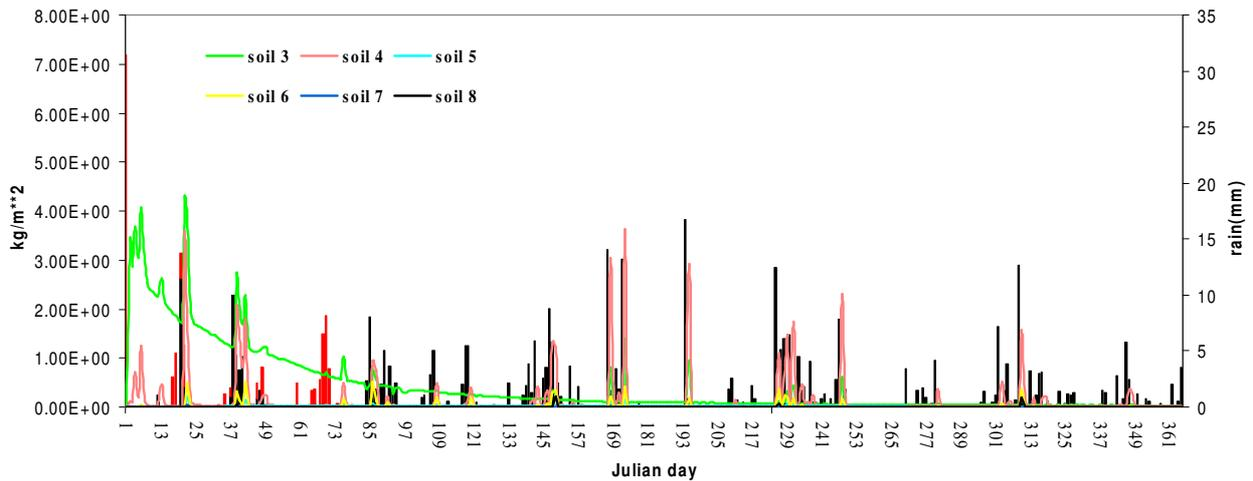
**graph 12:** the black bar represents the cumulated daily precipitations and the red bar represents snow precipitation; the others curves are the subsoil runoff curves varying the soil type
