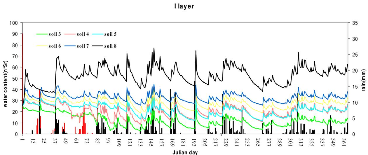
**graph 3:** the black bar represents the cumulated daily precipitations and the red bar represents snow precipitation; the others curves are the water content curves in the first soil level varying the soil type
