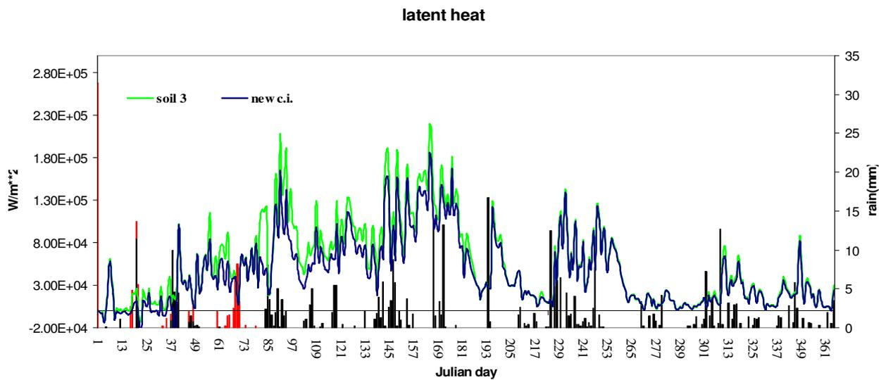
**graph 25 :** the black bar represents the cumulated daily precipitations,the red bar represents the snow precipitation; the others bars are the latent heat curves varying the initial conditions (green line for old i.c., blue for new i.c)
