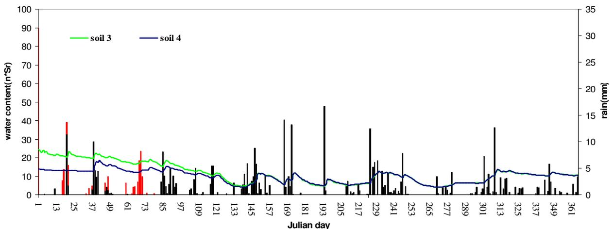
**graph 21 :** the black bar represents the cumulated daily precipitations, the red bar represents the snow precipitation; the others bars are soil moisture curves in the IV layer varying the initial conditions (green line for old i.c., blue for new i.c)
