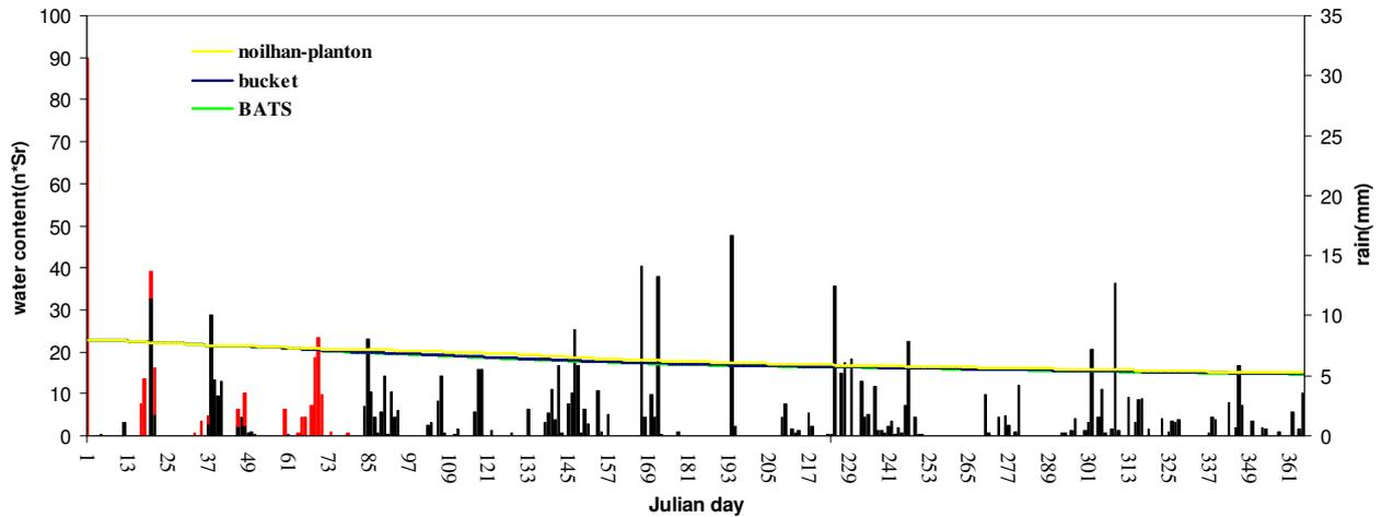
**graph 15:** the black bar represents the cumulated daily precipitations, the red bar represents the snow precipitation; the others bars are the soil moisture curves in the VI layer varying the evaporation model (green line for BATS model, yellow line for Noilhan-Planton model and blue for bucket model)
