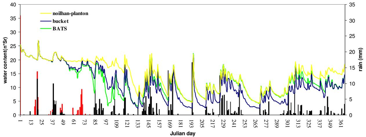
**graph 13:** the black bar represents the cumulated daily precipitations, the red bar represents the snow precipitation; the others bars are the soil moisture curves in the I layer varying the evaporation model (green line for BATS model, yellow line for Noilhan-Planton model and blue for bucket model)
