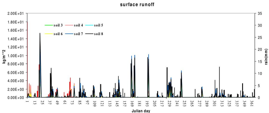
**graph 11:** the black bar represents the cumulated daily precipitations and the red bar represents snow precipitation; the others curves are the surface runoff curves varying the soil type
