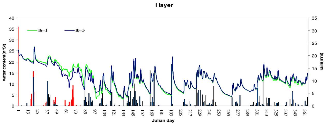
**graph 28**: the black bar represents the cumulated daily precipitations; the red bar represents the snow precipitation; the others bars are the soil moisture curves in the first layer varying the lower boundary (green line for the unit gradient condition and blue for constant groundwater condition)
