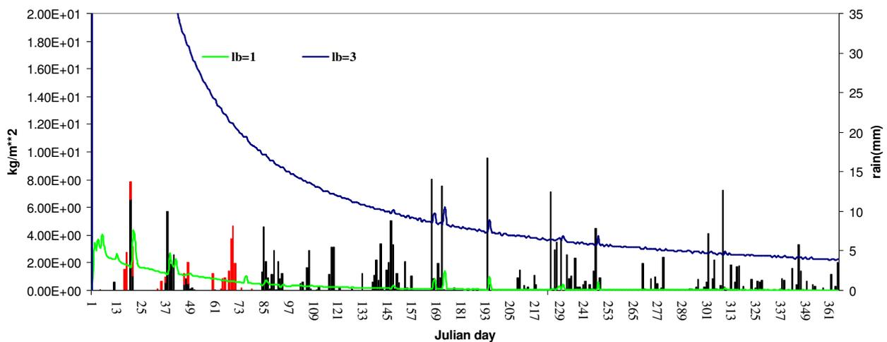
**graph 33:** the black bar represents the cumulated daily precipitations; the red bar represents the snow precipitation; the others bars are the subsoil runoff trends varying the lower boundary (green line for the unit gradient condition and blue for constant groundwater condition)
