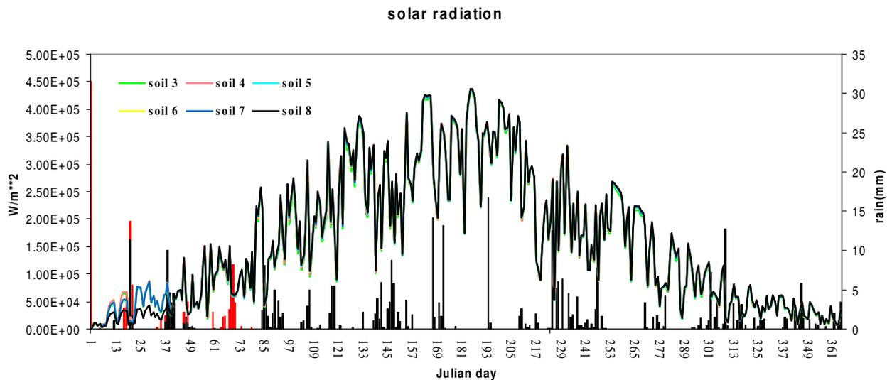
**graph 10:** the black bar represents the cumulated daily precipitations and the red bar represents snow precipitation; the others curves are the solar radiation curves varying the soil type
