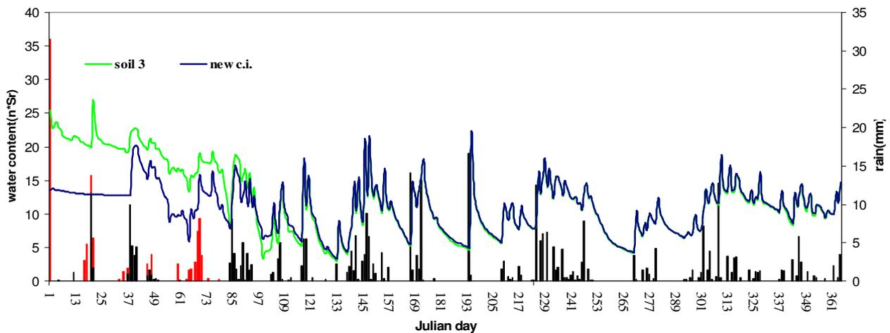
**graph 20:** the black bar represents the cumulated daily precipitations, the red bar represents the snow precipitation; the others bars are soil moisture curves in the I layer varying the initial conditions (green line for old i.c., blue for new i.c)
