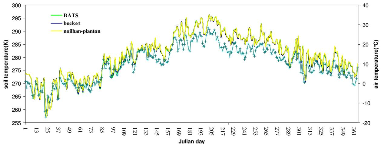
**graph 16:** the grey curve with the crosses represents the air temperature, the others bars are the soil temperature curves in the III layer varying the evaporation model (green line for BATS model, yellow line for Noilhan-Planton model and blue for bucket model)
