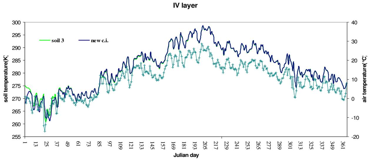
**graph 24:** the grey curve with the crosses represents the air temperature; the others bars are the soil temperature curves in the IV layer varying the initial conditions (green line for old i.c., blue for new i.c)
