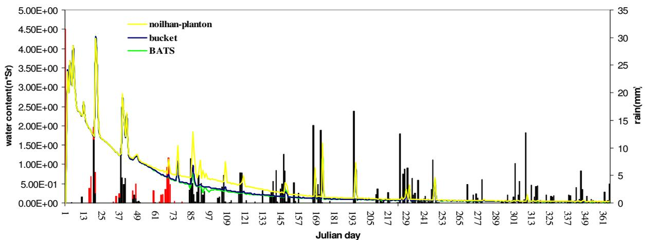
**graph 19:** the black bar represents the cumulated daily precipitations, the red bar represents the snow precipitation; the others bars are the subsoil runoff curves varying the evaporation model (green line for BATS model, yellow line for Noilhan-Planton model and blue for bucket model)
