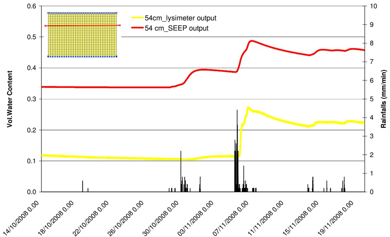
Fig.10 Water content trends at 54cm from the lysimeter' s bottom
