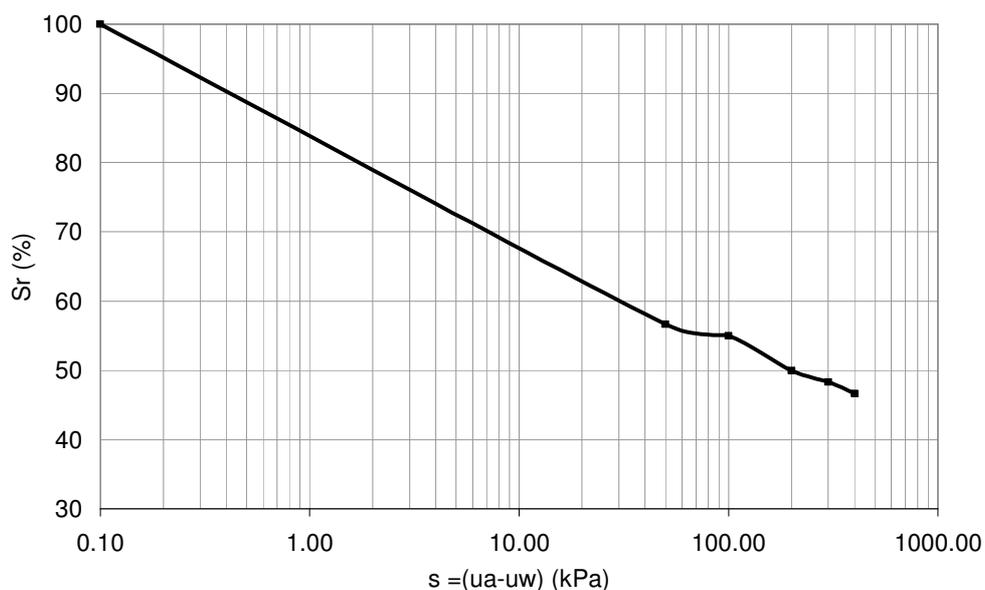
*Fig.5 Volumetric water content function*
