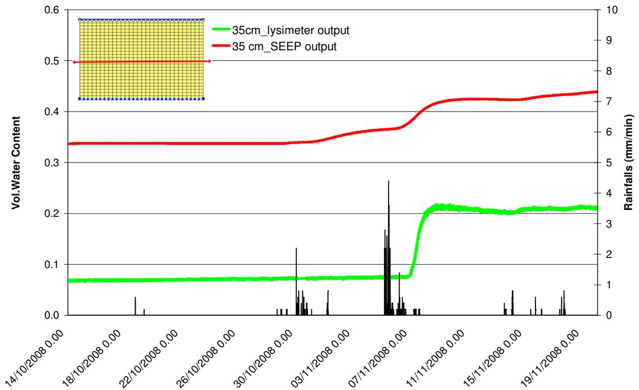
Fig.11 Water content trends at 35cm from the lysimeter's bottom
