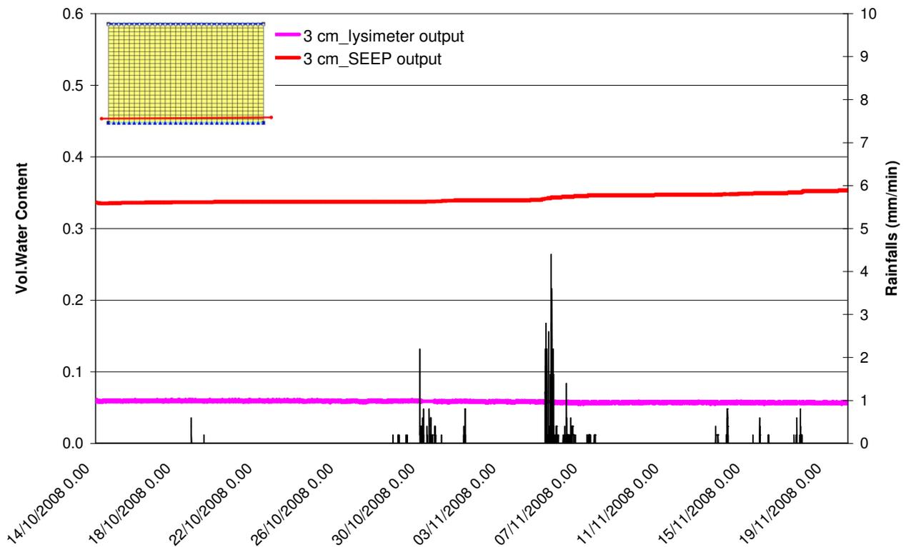
*Fig. 13 Water content trends at 3 cm from the lysimeter' s bottom*
