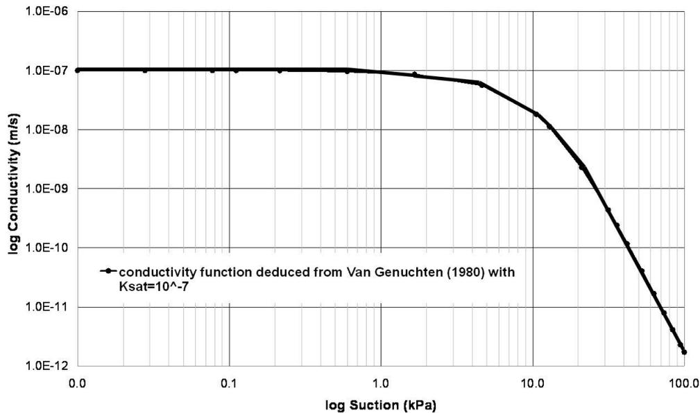
Fig.6 Hydraulic conductivity function
