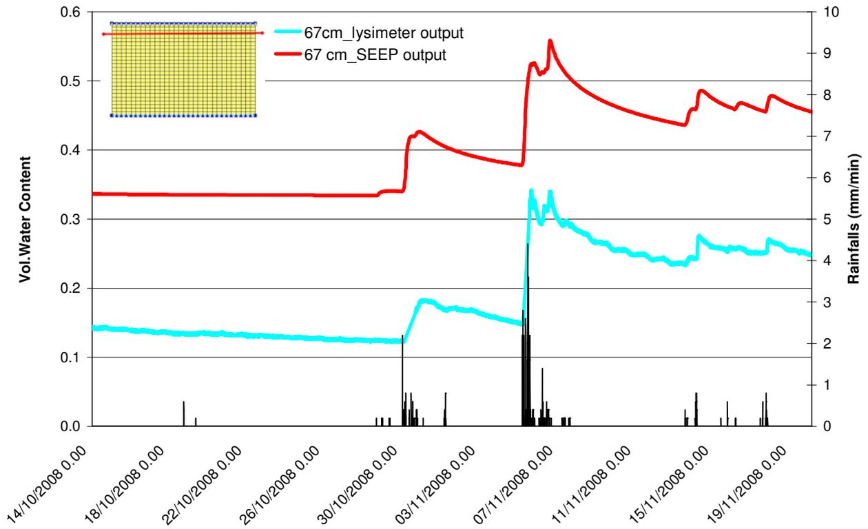
Fig.9 Water content trends at 67cm from the lysimeter' s bottom
