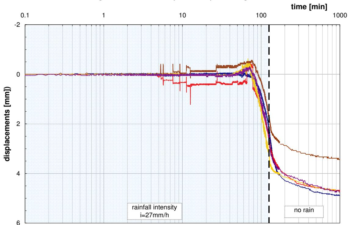
Figure 19. Test on layered slope – Stage II: settlement of ground surface
