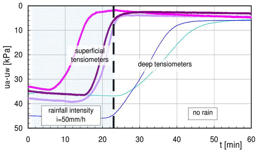
Figure 7. Suction against time during test D9\_1
