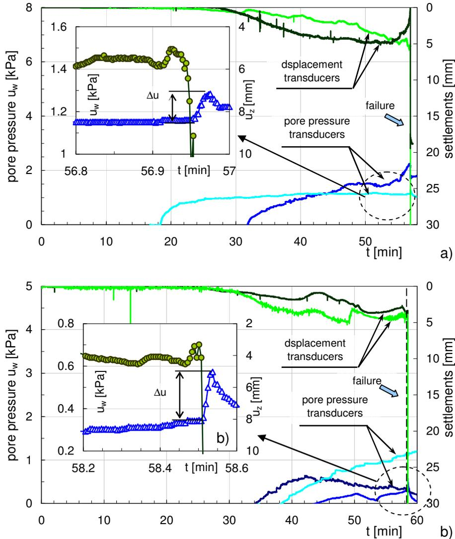
Figure 11. Pore pressures at the base of model slope during: a) test D9-2; b) test D10-2
