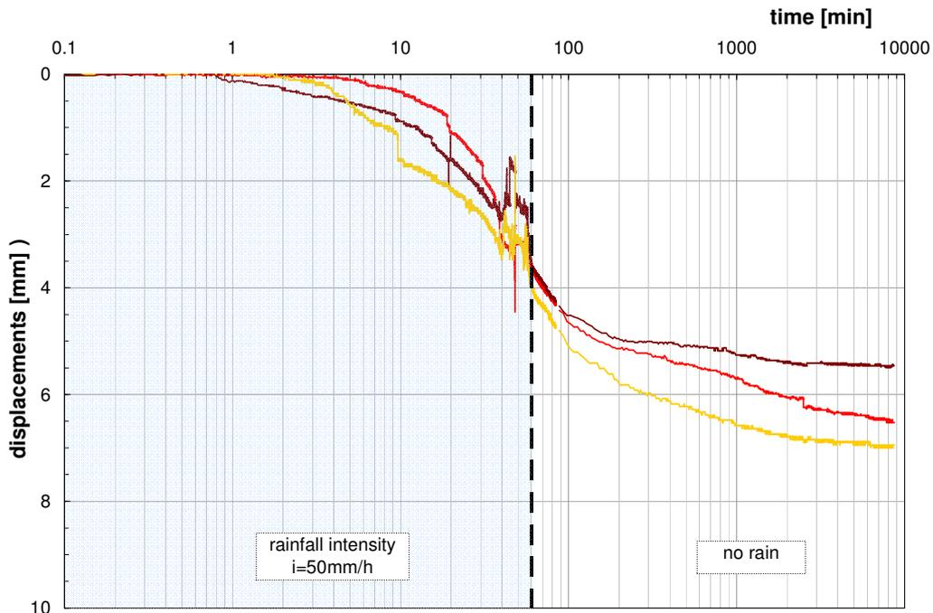
Figure 17. Test on layered slope – Stage I: settlement of ground surface
