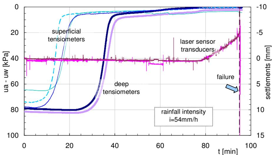
Figure 5. Suction and settlement of the ground surface against time during test D7
