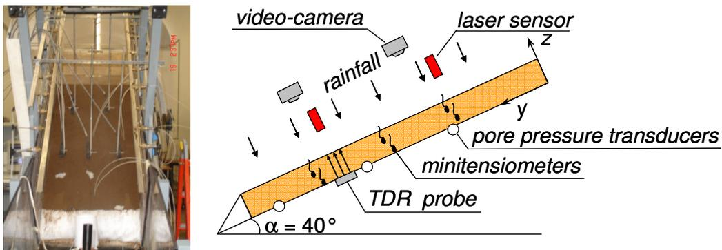
Figure 3. The instrumented flume
