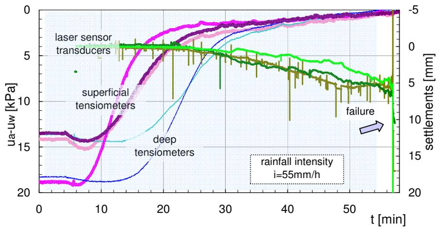
Figure 8. Suction against time during test D9\_2
