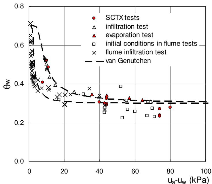
Figure 13. Cervinara volcanic ash: Water Retention Curves obtained from infiltration tests and conventional long-term laboratory tests (Olivares and Tommasi, 2008).
