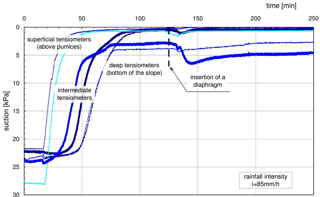
Figure 21. Test on layered slope – Stage V: suction against time
