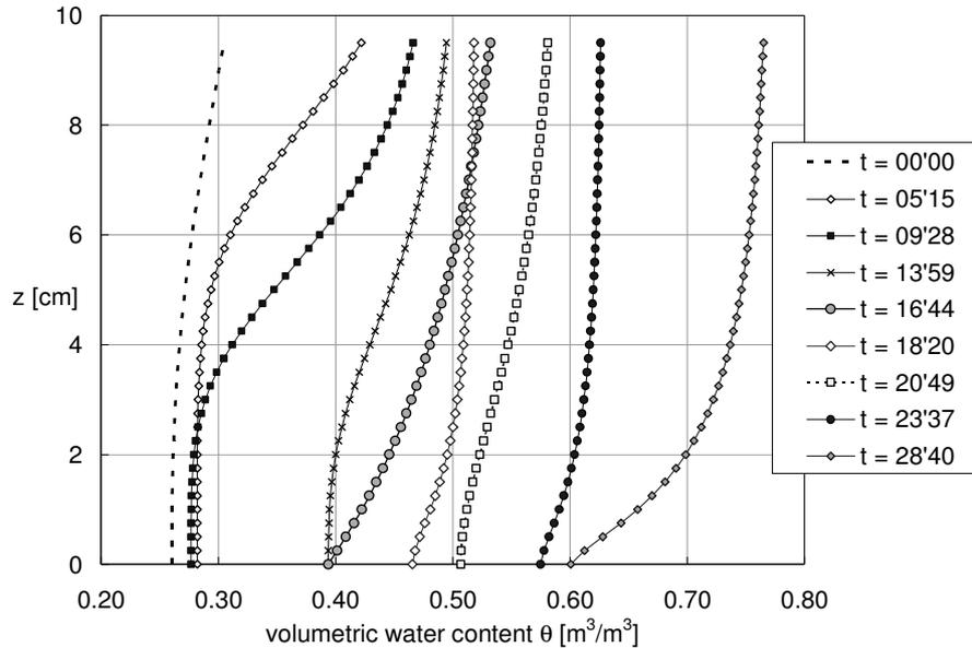
Figure 12. Volumetric water content profiles at different times during test D4 (Damiano et al., 2008)
