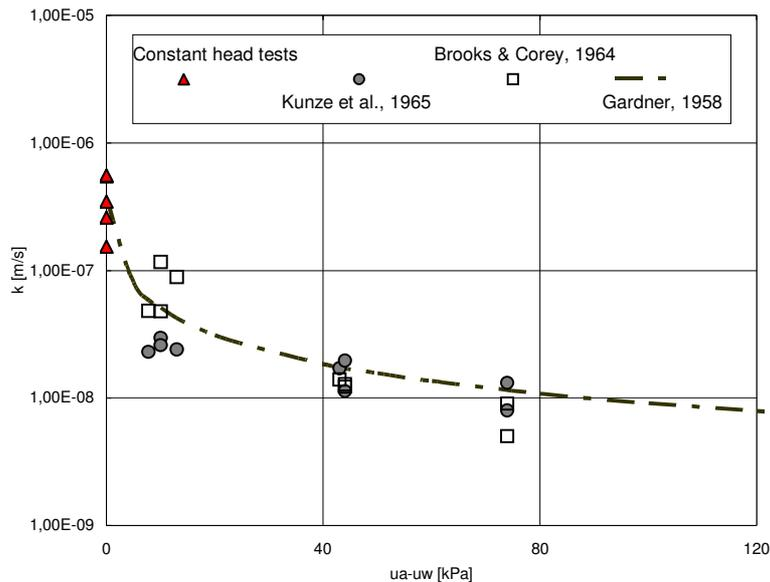
Figure 2. Unsaturated permeability on Cervinara volcanic ashes (Picarelli et al., 2006).
