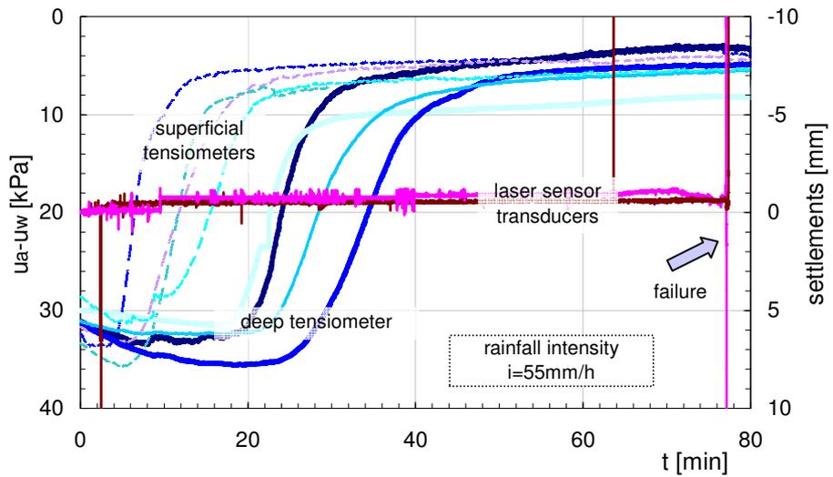
Figure 6. Suction and settlement of the ground surface against time during test D8
