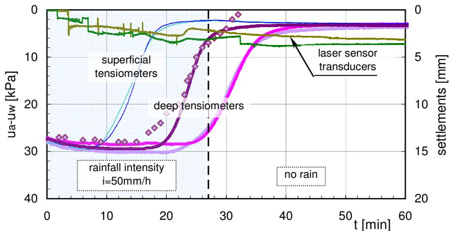
Figure 9. Suction and settlement of the ground surface against time during test D10\_1
