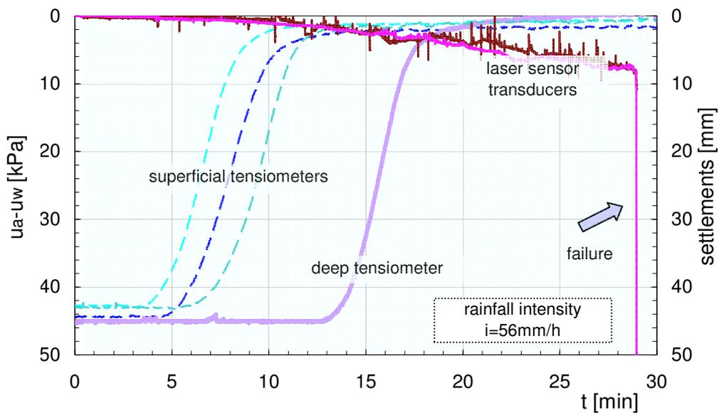
Figure 4. Suction and settlement of the ground surface against time during test D4
