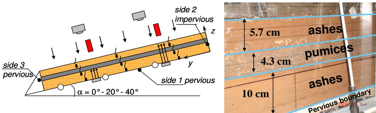
Figure 15. Sketch of test on layered small-scale slope and side-view of the soil deposit.
