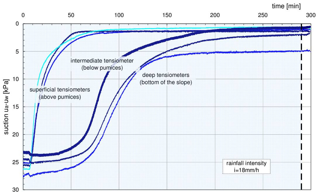
Figure 20. Test on layered slope – Stage IVa: suction
