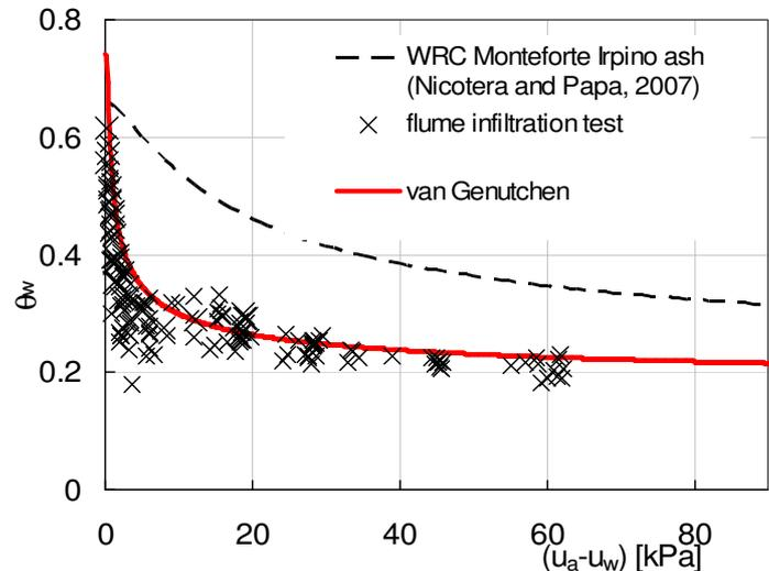
Figure 14. Monteforte Irpino ash: Water Retention Curve obtained from infiltration tests and conventional long-term laboratory tests (Nicotera and Papa, 2007).
