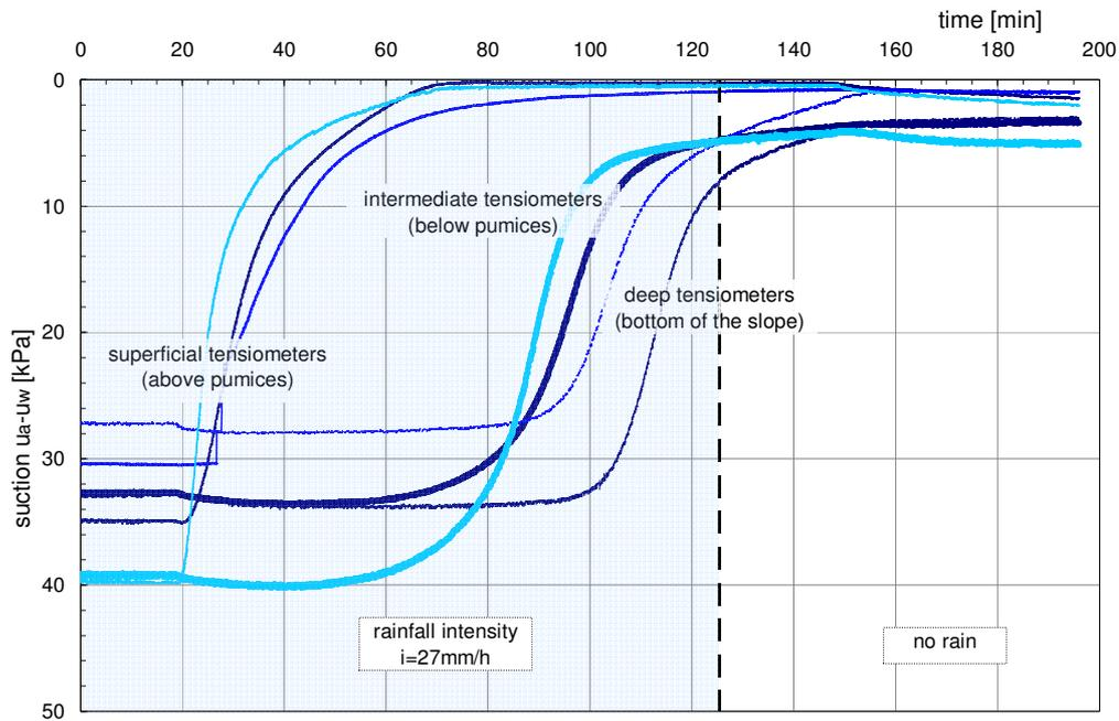
Figure 18. Test on layered slope – Stage II: suction
