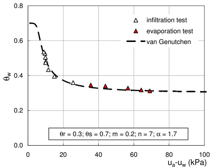
Figure 1. Soil Water Retention Curve of Cervinara volcanic ash from conventional tests.
