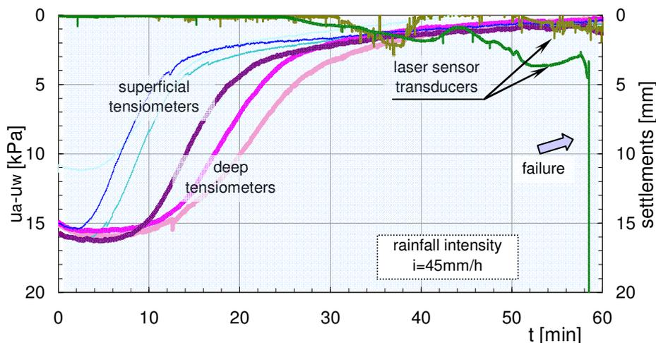
Figure 10. Suction and settlement of the ground surface against time during test D10\_2
