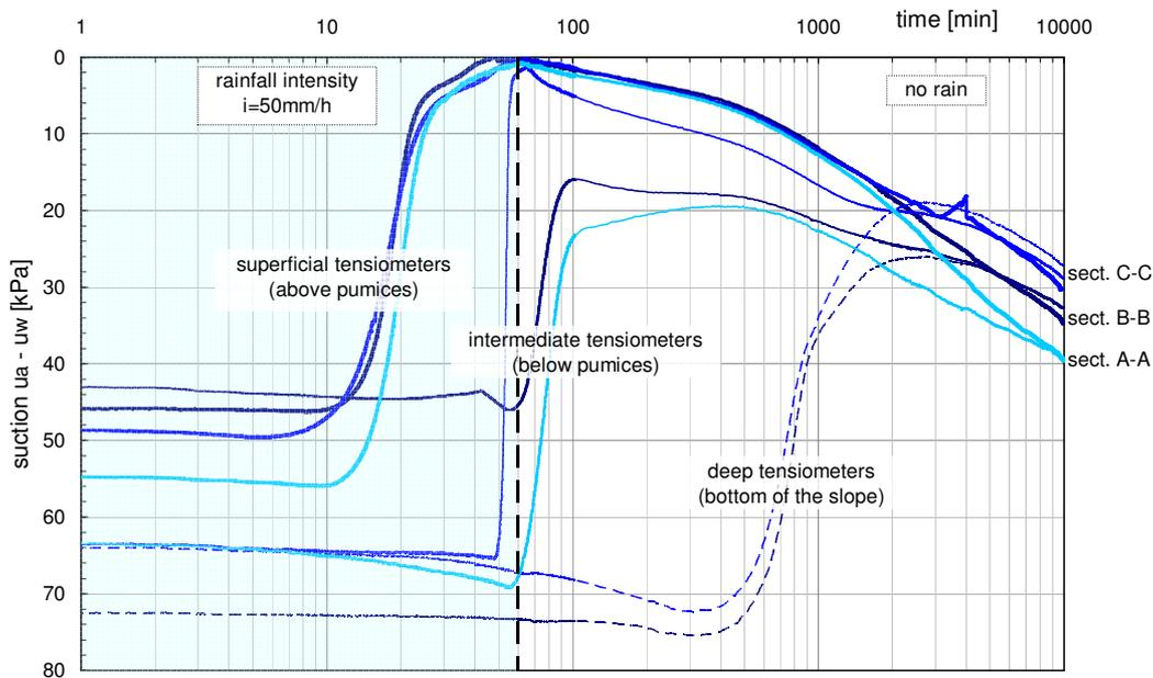
Figure 16. Test on layered slope – Stage I: suction
