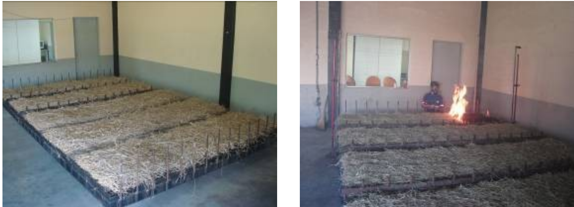
Figure 2. The LCI–Rio Sagrado Fire Lab showing the main combustion bed.
