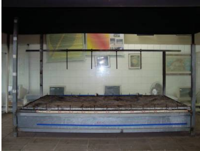
Figure 1. The UFPR Fire Lab combustion chamber and the fuel bed.
