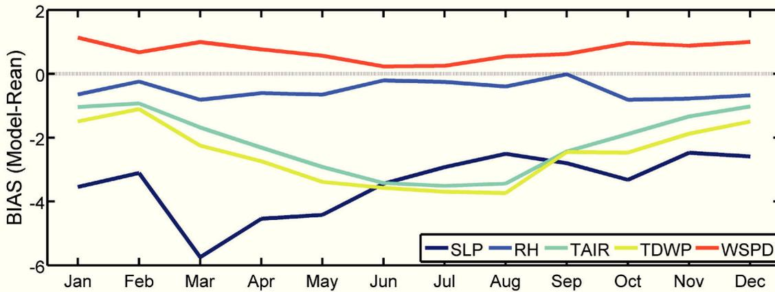
**Figure 2.** Time series of the difference between the CMCC-CM and ERA-Interim monthly climatologies over the Mediterranean basin for the period 1979-2010. Variables in the plot: SLP - sea level pressure (hPa); RH – relative humidity (%); TAIR – Air temperature at 2 m (°C); TDWP – Dew Point temperature at 2m (°C); WSPD – Wind speed module (m/s). Positive values indicate an overestimation of the CMCC-CM data with respect to ERA-Interim Reanalyses.
