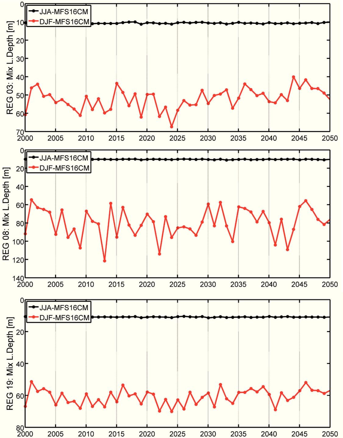
**Figure 10.** Time series of summer (JJA) and winter (DJF) seasonal Mixed Layer Depths of the scenario MFS16 simulation (MFS16CM) for the Provencal basin (top, Reg. 3), Ionian Sea (middle, Reg. 8), and the whole Mediterranean Sea (bottom, Reg. 19). The spatial domain of each region is illustrated in Fig. 1.
