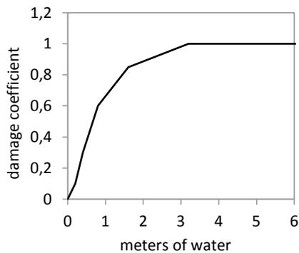
Figure 5: the water depth-duration curve of productivity loss considered in this study.
