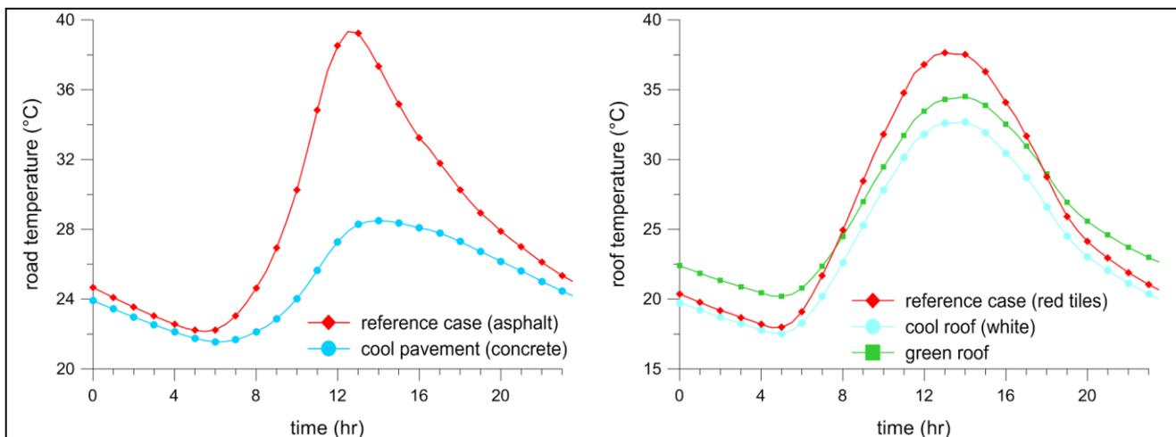
Figure 2: Summer average diurnal cycle of road temperature (left) and roof temperature (right) for different adaptation strategies.
