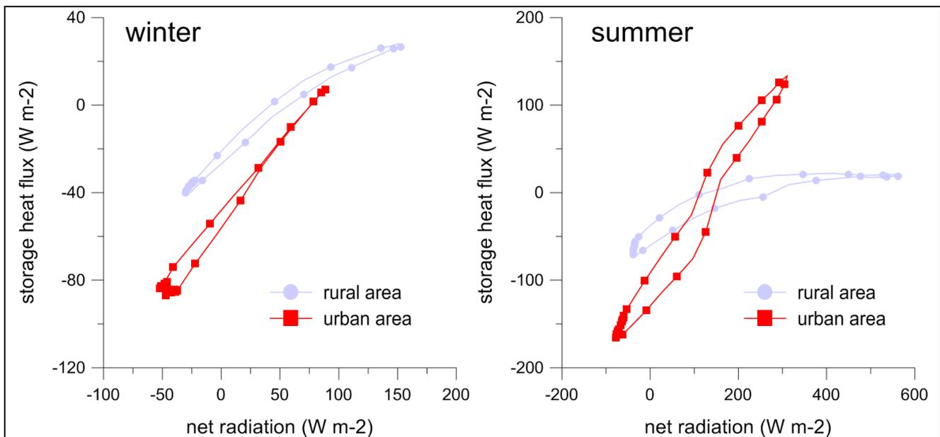
Figure 1: Comparison of energy cycles (net radiation against storage heat flux) for urban and rural areas during winter and summer (positive values of storage heat flux represent a flux warming the surfaces of the urban elements; negative values of storage heat flux tends to warm the canyon).
